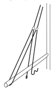
To find the boom positions, first identify your boom length (E measurement on your sail plan). The two aft eyes (No 2) should be positioned between 70% and 80% of this measurement. The forward eye and cheek block (No 3) should be positioned between 30% and 40% of the boom length.
