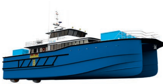
Wind service support vessel with Voith Linear Jet
