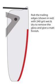
File half the trailing edge thickness to a 45 deg bevel. Do this on the inside of the foils so the bevels on opposite foils are face each other.
