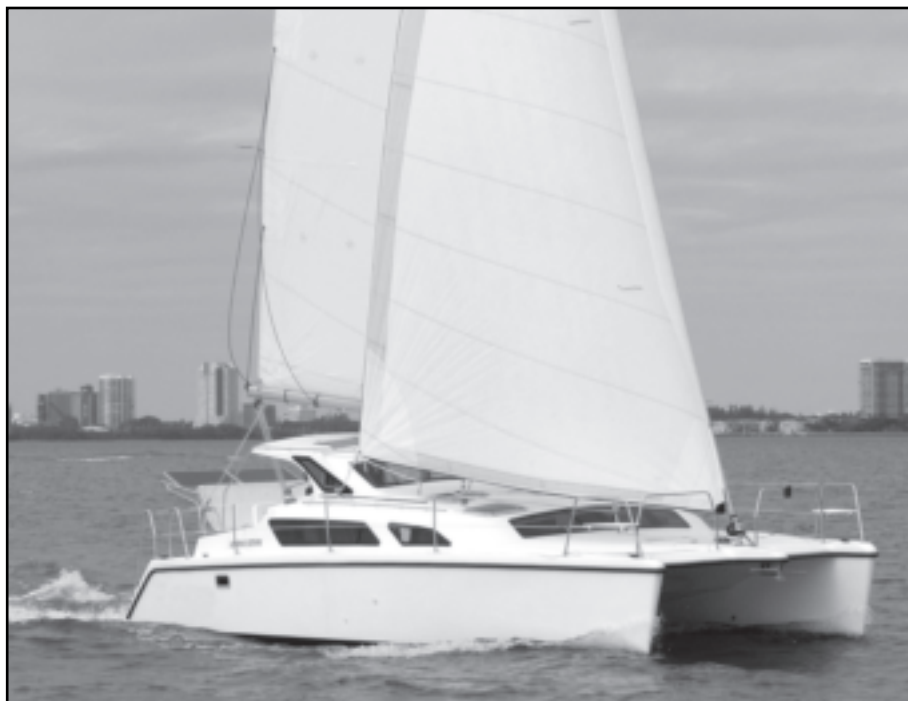
The Gemini 105Mc shows a good turn of speed off Miami. Note the solar panels rigged on the davits, and the drop-through anchor platform. This boat isn't rigged with the optional track forward for shifting the screecher tack athwartships.
