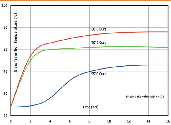
When curing a composite part, the whole of the part (including the very middle of the laminate) needs to see the cure temperature.
