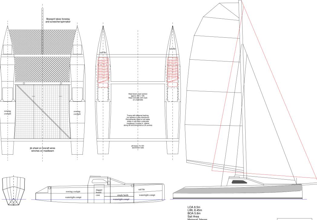
LWL 8.45m BOA 5.8m Sail Area Mainsail 34sqm Jib 16sqm (screecher in red 38sqm) Empty weight 700kgs Displacement to WL 990kgs Draft 250, (1200 boards down) 2 single berths in hulls headroom 1.75m
