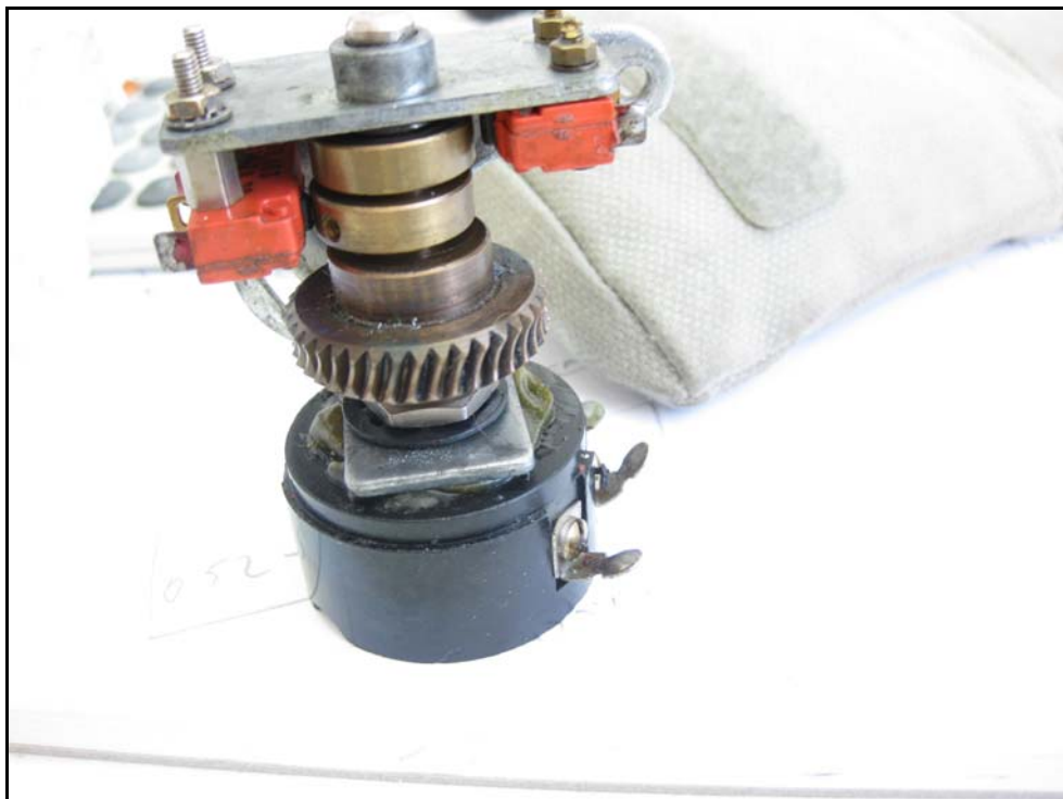
Figure 6. Neco rudder feedback and “end-switches” assembly (photograph by N.Kassel).
