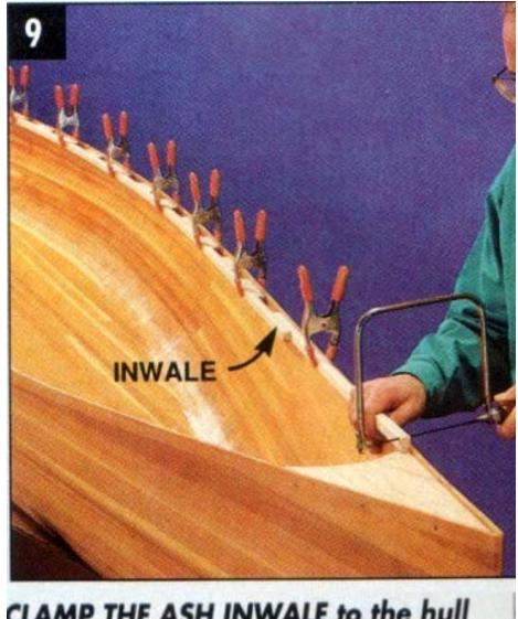
CLAMP THE ASH INWALE to the hull 1/4 in. below the edge, and trim one end to fit. Screw the inwale to the hull, then trim the other end.
