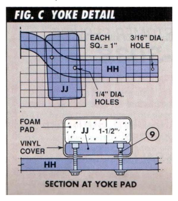
Clamp the yoke to the undersides of the inwales with two small C-clamps. Set the canoe on your shoulders and see how it balances. Adjust the yoke forward or backward on the inwale until the canoe balances perfectly, then drill the yoke bolt holes and bolt it in place.
