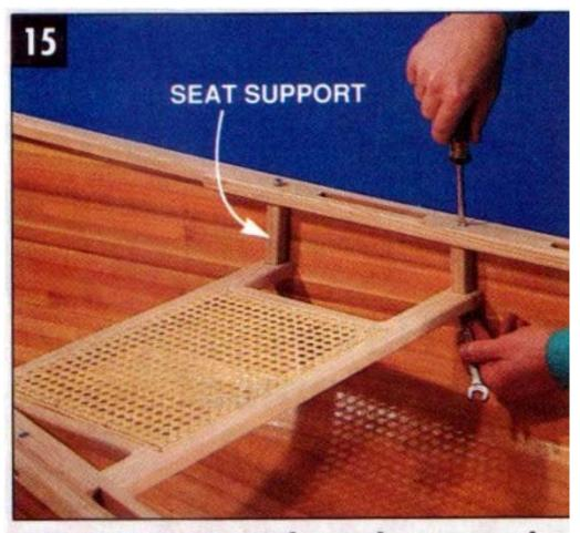
HANG THE SEATS from the gunwales with long bolts and seat support blocks. The front edge of each seat is hung lower for paddling comfort.
