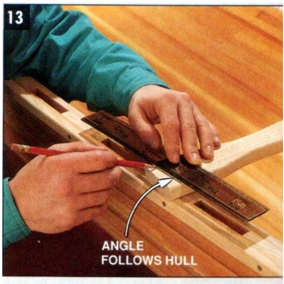
MARK THE THWARTS so they fit the angle of the hull, cut them, then bolt them on underneath the inwales with stainless steel bolts.
