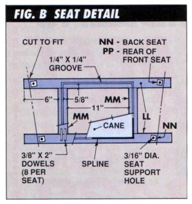
The prewoven cane seat is attached as follows: (1) Rout a  $1/4 \times 1/4$ -in. groove in the tops of the seat frame, using a straightedge to guide the router when cutting the rails (Photo 14);
