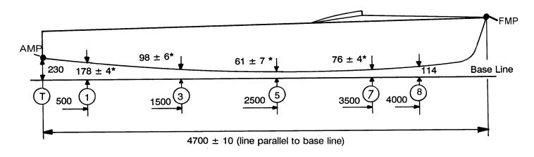
8.3 To check the profile of the keel a base line shall be fixed at 230mm below the lowest point of the transom and 114mm below the keel at section 8. The distance between the base line and keel shall not differ from the figures on the measurement diagram by more than 4mm at station 1 and 7, 6mm at station 3 and 7mm at station 5, and the algebraic differences of the maximum positive and maximum negative deviations shall not exceed 10mm.
