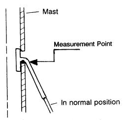
11.11 The measurement point of a hammerhead shroud fitting will be as shown.
