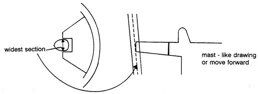
meet this requirement the widest section of the mast shall be within the mast partners when the forestay is under tension.
