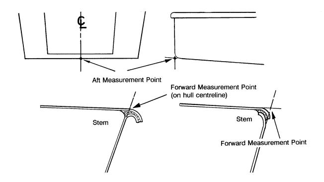
8.2 Measurement sections, transom, 1, 3, 5, 7, and 8 shall be at 0mm, 500mm, 1500mm, 2500mm, 3500mm and 4000mm respectively from the Aft Measurement Point on the transom.
