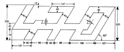
(b) (i) The mainsail shall carry the national letters and sail number in red. They shall be placed as shown in the diagram and shall be of the following minimum dimensions:
