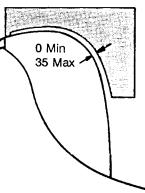
with the hull shell) shall be verified at the transom (580mm), at section 4 (830mm), and at section 6 (770mm) with a tolerance of  $\pm$  30mm.
