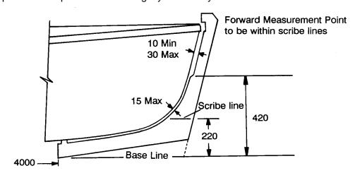
8.5 Templates for the transom and section 1, 3, 5, 7 and 8 shall be applied as shown on the measurement diagram. The top of the deck at the sheerline shall not be more than 10mm above or below the sheer marks on the templates. The templates shall touch the gunwale rubbing strakes lightly or clear by not more than 35mm. At the transom the distance to the template shall be defined as shown in the diagram.
