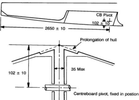
Edge of template located at inner edge of wooden rubbing strake. Where there is no wooden rubbing strake, a point 30mm from the outer edge shall be used.
