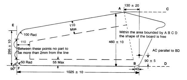
(ii) The shape of the lower corners shall be not more than 10mm from the designed shape.
