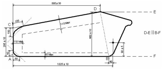
The contour of the centreboard is defined by the points A, B, C, D and the lines DE and BF.
