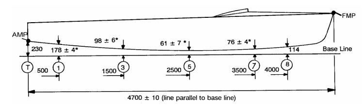
8.3 To check the profile of the keel a base line shall be fixed at 230mm below the lowest point of the transom and 114mm below the keel at section 8. The distance between the base line and keel shall not differ from the figures on the measurement diagram by more than 4mm at station 1 and 7, 6mm at station 3
