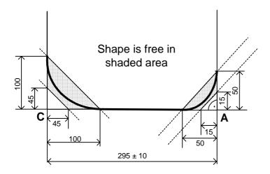
10.4 The rudder shall be of even thickness throughout 22mm  $\pm$  2mm, except that the edges may be reduced as defined in rule 10.5. Except for permitted reducing the thickness shall not vary by more than 1mm.
