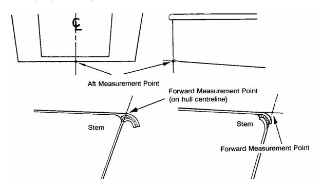
8.2 Measurement sections, transom, 1, 3, 5, 7, and 8 shall be at 0mm, 500mm, 1500mm, 2500mm, 3500mm and 4000mm respectively from the Aft Measurement Point on the transom.
