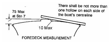
not be more than 10mm above or below the sheer marks on the templates. The templates shall touch the gunwale rubbing strakes lightly or clear by not more than 35mm. At the transom the distance to the template shall be defined as shown in the diagram.
