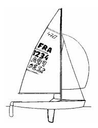
6.4 Mainsails and headsails shall carry the official **certification mark** near the tack point and spinnakers shall carry the official **certification mark** near the **head point**.
