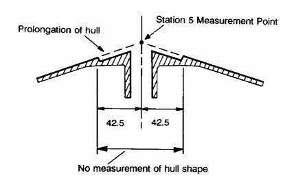
8.4 The stem template shall be applied as shown on the measurement diagram. Between the sheerline and a point 420mm above the baseline the template shall clear by not less than 10mm nor more than 30mm. Below the 420mm point the template shall touch lightly or clear by not more than 15mm.
