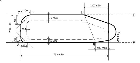
The contour of the rudder blade is defined by the points A,B,C,D and the lines DE and BF.
