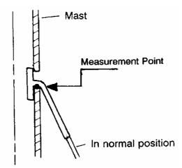
11.11 The measurement point of a hammerhead shroud fitting will be as shown.
