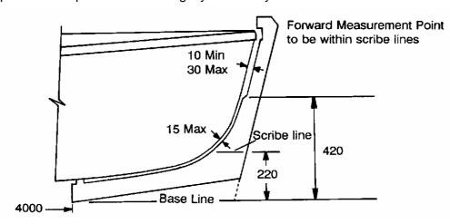
8.5 Templates for the transom and section 1, 3, 5, 7 and 8 shall be applied as shown on the measurement diagram. The top of the deck at the sheerline shall
