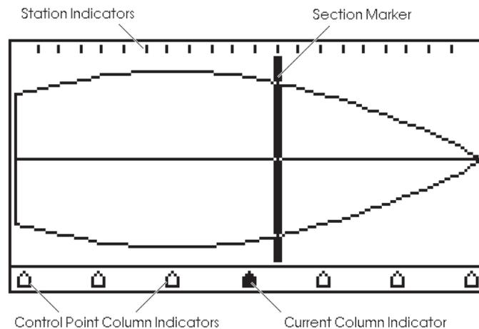
At the top of the control box several short vertical lines are drawn. These are the station indicators; there is one indicator for each of the stations specified in the Design Grid dialog.
