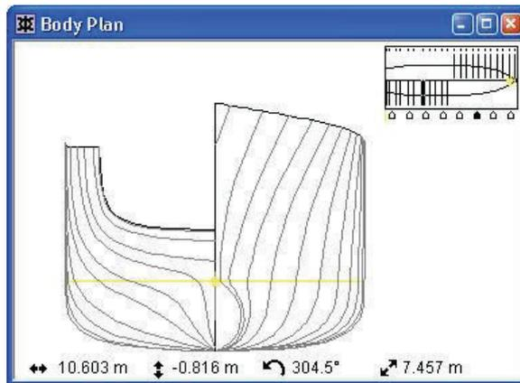
If Split Section Display is not chosen, all stations will be drawn over half of the hull on the right hand side of the centreline.
