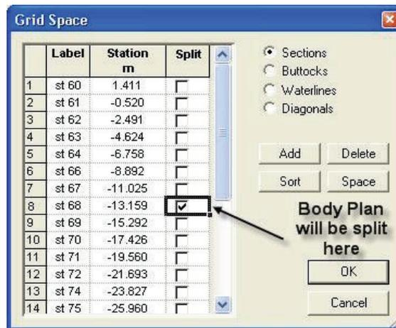
The Control box in the body plan window will be drawn with the sections staggered to show where the split has been placed:
