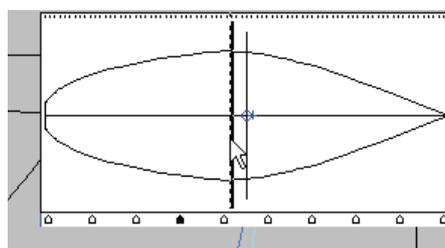
By clicking at the desired longitudinal position well inside the control box, the section closest to that longitudinal position is displayed. By using the arrow keys on your keyboard you can then scroll through the sections. The right arrow displays the next station forward and the left arrow displays the next station aft.
