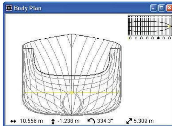
When the Half function is not activated, both sides of each symmetrical surface will be displayed. However, when Half is activated, the Body Plan window will show either a split section view or all sections on one side depending on whether Split Section Display is setup correctly. The Split Section Display option is described in greater detail in the next section.
