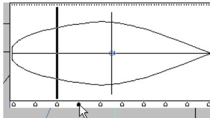
By selecting the triangles you select a column of control points and display the section that is closest to that column. Alternatively, a column is made the current column of its respective surface whenever one of its control points is selected in any of the drawing windows.
