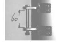
Put on the endless rollerreefingline with the 3-disk-block around the selftailing head at the front of the rollerreefingboom.
