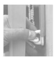
Put the sliders again in the masttrack when hoisting the profile.
