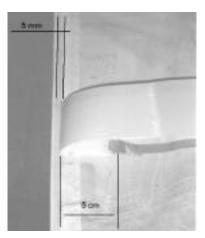
to the batten-pocket-strip. On the sail you stitch a 10 cm long and approx.4 cm wide strip of **velcro-hook** placed so that it will fall under the battenpocket-strip end.
