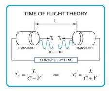
For example, if the wind blew from the north, time of ultrasonic from N to S will be shorter than from S to N, and transmission time of it from W to E and E to W is the same. Through calculating the time difference of ultrasonic transmission between two points, the wind speed and direction can be calculated. This calculation
