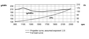
Test conditions Air temperature +25°C. Barometric pressure 100 kPa (750 mmHg). Humidity 30 %. Diesel fuel acc. to ECE R 24 Annex 6. Density of fuel 0.840 kg/dm³. Viscosity of fuel 3.0 cSt at 40°C. Energy value 42700 kJ/kg. Power test code ISO 3046. Power and fuel values +/-3%.
