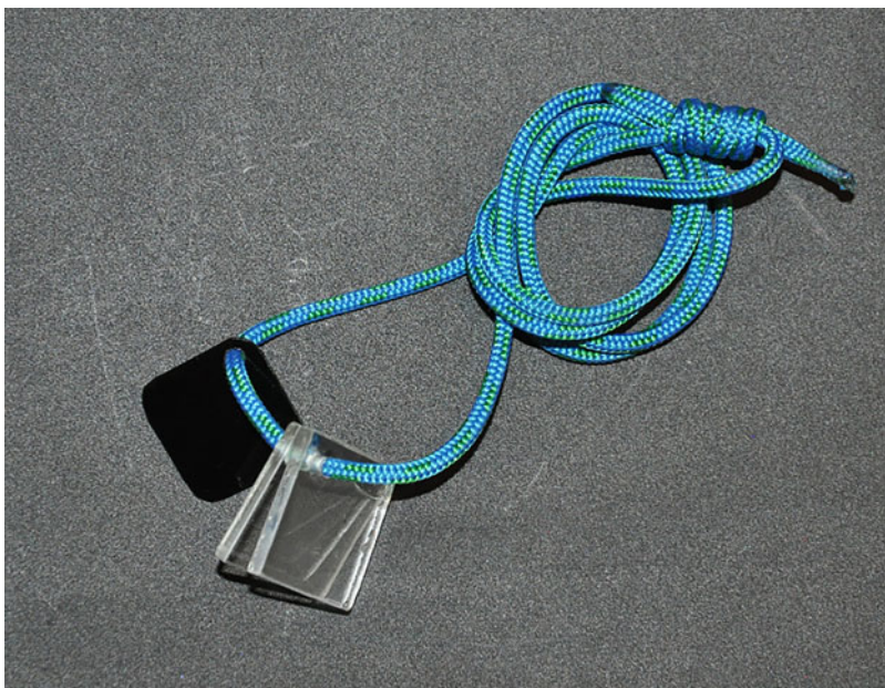
Figure 1. A Bris sextant. This is a simple model with only two panes of glass, drilled to be carried on a lanyard around the neck (for quickly checking the Sun). In this case, greater refraction is made possible with the use of teleprompter-type glass which makes more of the light refract rather than pass through. Note that this model also has a shade-5 welding filter on the lanyard to prevent the brighter images from damaging the viewer's eyes. Higher images, which are only refracted a few times, can be quite bright, whereas lower images are dimmer.
