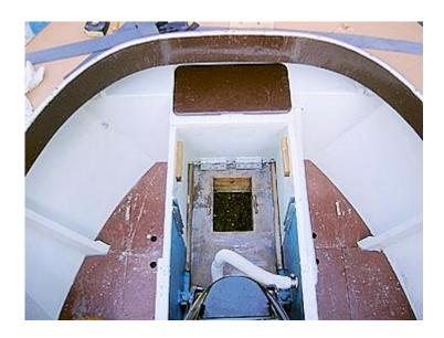
The aft portion of the motor well has a thick swing up/removable plug. The aft bottom sections of Bartenders are narrow to preserve the pointy stern for following seas. To gain planning surface George Calkins designed this nifty motor well plug. The smaller cut out is removable mini plug that one can put a small outboard -- 4 hp. or so. This motor would be used in an emergency or to troll while fishing.
