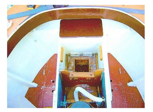
Right: The portable transom for the small outboard is in place.
