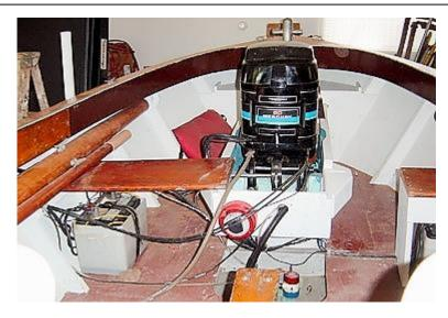
Looking into the aft portion of the cockpit shows the 50 hp. Mercury outboard and a split bench seat with batteries under. The exposed bilge pump rests at the below the motor well splash pan.
