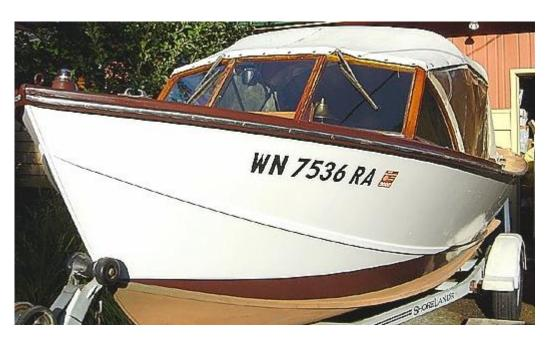
Another characteristic of Bartenders is the sprayrails. The upper rail terminates below and parallel to the waterline. Just before the stern it widens (see above) forming additional surface area allowing the boat to get on a plane faster.
