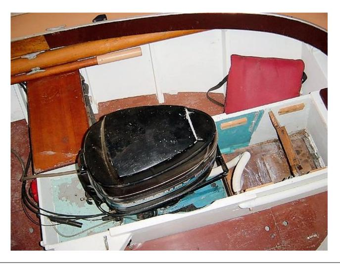
Looking down into the motor well note the white pipe hooked to the Merc's exhaust outlet. The pipe continues to the outside of the well, turns aft and exits out the stern. At slower speeds, these engines exhaust out below the power head. Only at higher speeds is all the exhaust directed to the thru-prop exit underwater.
