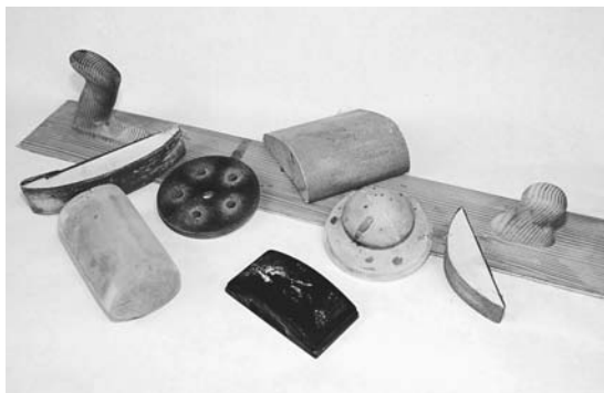
Figure 3-5. Hand sanding is always a part of strip-planking boats. A good sanding block is essential to fast, efficient work. I use the round unit on the right with “used” disks off my random orbit power sander. The round pad on the left is a soft foam conforming adapter for use with the power sander or hand sanding pad. The standard rubber sanding block at the lower center works very well with sheet sandpaper. I also wrap sheet paper around the chunk of foam to get at inside surfaces. Sandpaper can be glued or stapled to different-shaped blocks of wood to fit curved shapes. Under all the other blocks is a shop-made “long-board” fairing sander. This quickly levels out uneven surfaces.
