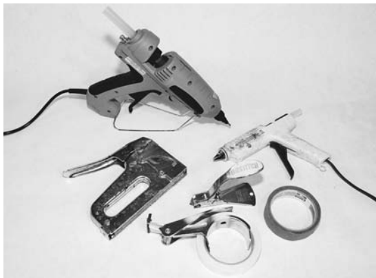
Figure 2-7. The strip planks need to be temporarily secured to the forms. The widely available T-50 utility staple on the lower left is the standard. I like the Bostich heavy-duty staple remover. It does a good job of pulling the staples without damaging the strips. If you prefer, hot-melt glue can be used instead of staples. The glue sticks are strong enough to hold the plank in place but weak enough to break when you are done. Masking tape or strapping tape also provides a good, quick, temporary clamp to hold together adjacent strips.
