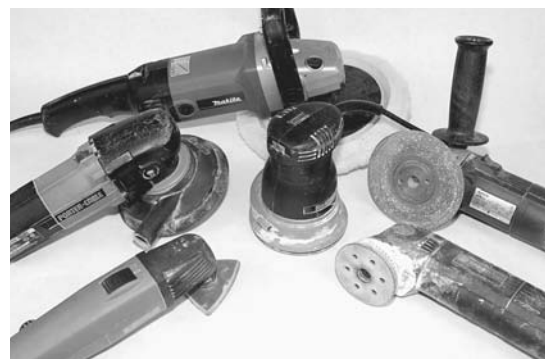
Figure 3-12. Power sanding saves a lot of time. The go-to tool is a random orbit sander, such as the middle unit, the larger one to its left, and the smaller detail sander at lower right. These remove material quickly with a minimum of sanding marks. The largest unit is the most powerful and the fastest, but it's hard to control; the small unit is good for small narrow pieces; and the middle unit is a good compromise. Above the smaller detail sander is a right-angle grinder. With very coarse sanding disks, this tool can remove a lot of material in a hurry. A detail sander is shown lower left, which occasionally is good for getting in tight spots. At top is an automotive polisher for buffing a finish.
